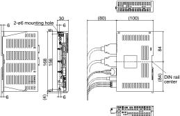
2-M5 screw Mounting screw Screw size: M5 Tightening torque: 1.87 [N·m] Mounting hole machining diagram
