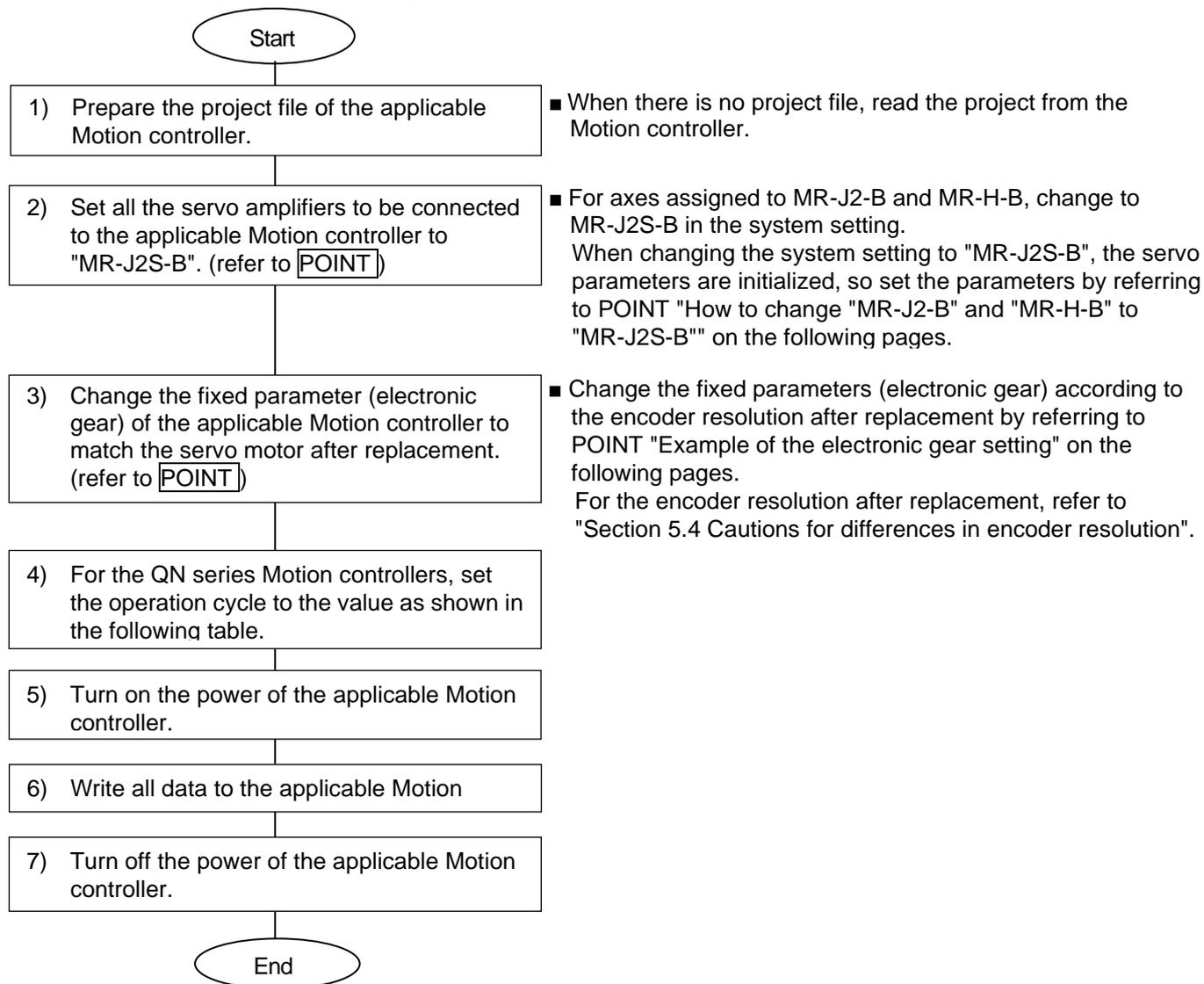
[QN series Motion controller (operating system software: SV13/SV22) operation cycle settings]
