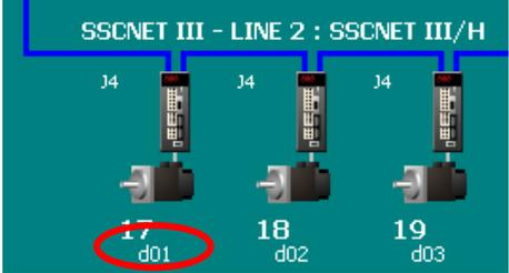
Axis number for the SSCNET III/H compatible servo amplifier
