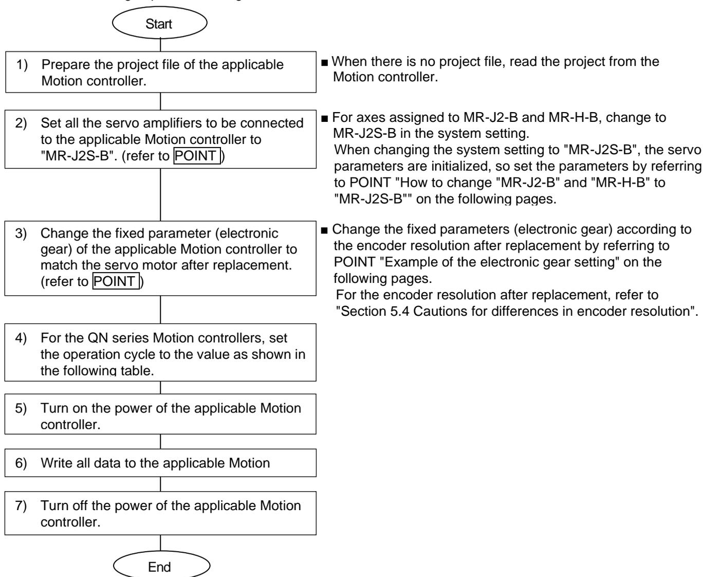
[QN series Motion controller (operating system software: SV43) operation cycle settings]
