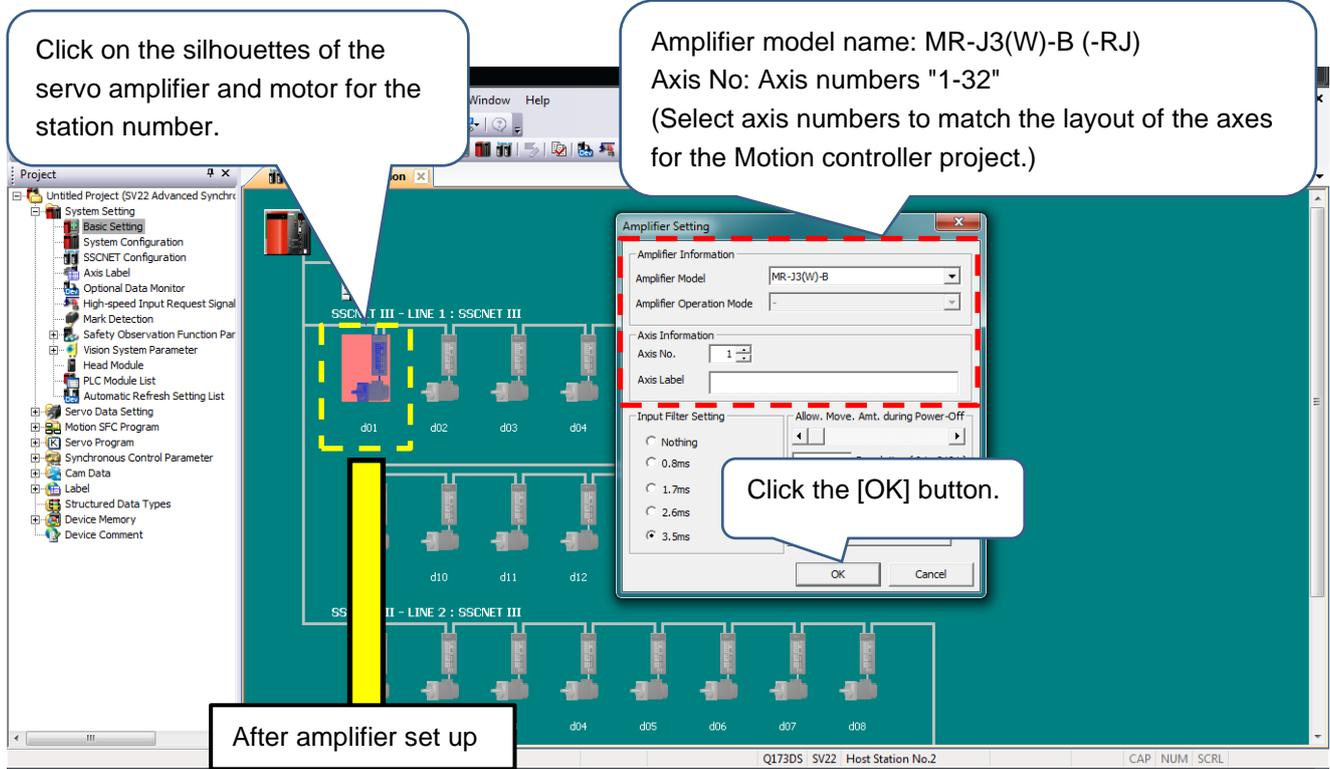
Click on the silhouettes of the servo amplifier and motor for the station number.
