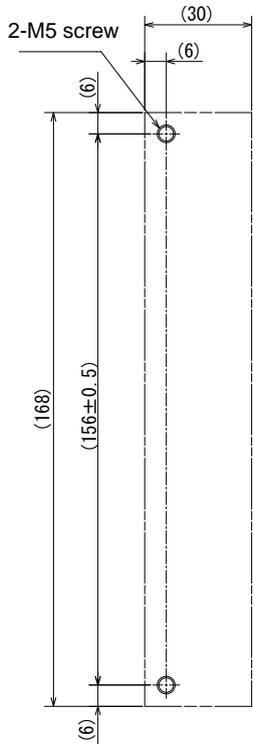
Mounting hole machining diagram
