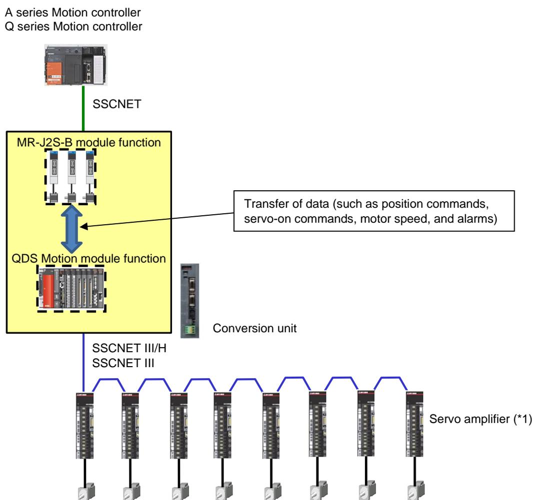
\*1: The SSCNET III/H compatible servo amplifiers are MR-J4-B/MR-J4W2-B/MR-J4W3-B, and the SSCNET III compatible servo amplifiers are MR-J4-B (J3 compatibility mode)/MR-J4W2-B (J3 compatibility mode)/MR-J4W3-B (J3 compatibility mode)/MR-J3-B/MR-J3W-B.
