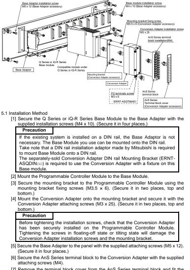
[7] Remove the terminal block cover from the AnS Series terminal block and fit the terminal block cover supplied with the Conversion Adapter in place.
