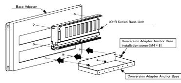
4.2 Installation without Base Adapter (Sold Separately) Screw hole machining (M4 × three positions) is required to mount the Conversion Adapter Anchor Base
