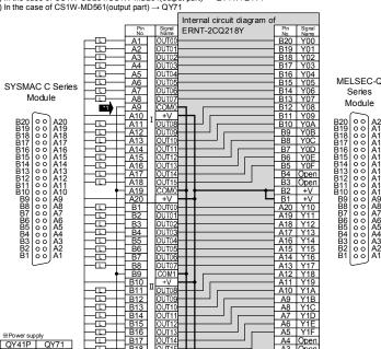
Because the switch concerned causes the number of points per common to change from 16 (two circuits) to 32 (one circuit), an alteration to the wiring is required if the commons on the existing nodules have been used in separation from each other.
