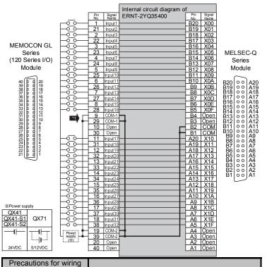
Because the switch concerned causes the number of points per common to change from 16 (two circuits) to 32 (one circuit), an alteration to the wiring is required if the commons on the existing modules have been used in separation from each other
