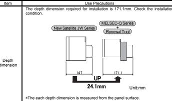
New Satellite JW Series: Base Unit + Input/output Module + Connector, MELSEC-Q Series + Renewal Tool: Base Unit + Input/output Module + Conversion Adapter + Connector
