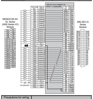
ecause the switch concerned causes the number of points per common to change from 16 (two circuits) to 32 (one circuit), an alteration to the wiring is required if the commons on the existing modules have been used in separation from each other.
