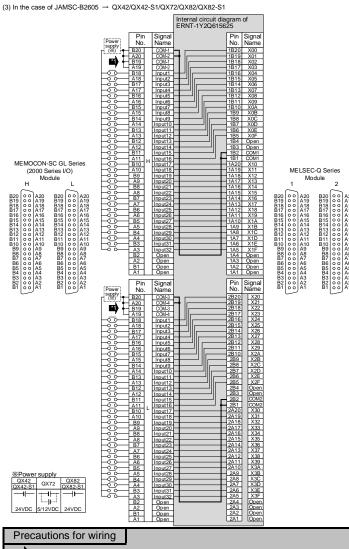
Because the switch concerned causes the number of points per common to change from 16 (four circuits) to 32 (two circuit), an alteration to the wiring is required if the commons on the existing modules have been used in separation from each other.
