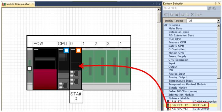
Set the starting XY address of the master/local unit of the second module to "0020".
