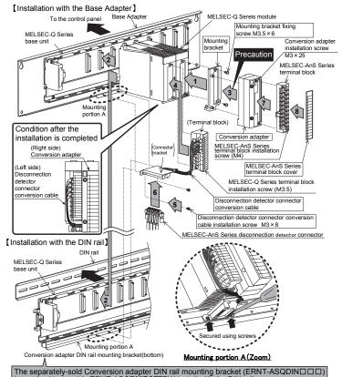
e separately-sold Conversion adapter DIN rail mounting bracket (ERNT-ASQDINDDD) equired to use this ERNT-ASQT62TCTTBW install with the DIN rail. For to the user's manual of the DIN rail mounting bracket of the Conversion Adapter for
