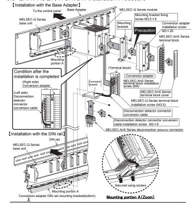
The separately-sold Conversion adapter DIN rail mounting bracket (ERNT-ASQDINDD) is required to use this ERNT-ASQT64TCRTBW install with the DIN rail.
