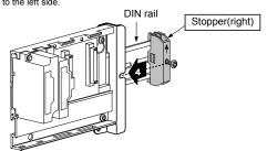
5. Penetrate the locking screw (M4 screw) of the stopper(right) through the opening of the Conversion Adapter DIN rail mounting bracket (right), then tighten the locking screw (M4 screw)
