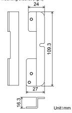
(2) Conversion Adapter DIN rail mounting bracket (bottom)
