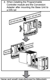
rail mounting adapter (large and small) manufactured by Mitsubishi Electric to the rear side of the MELSEC-Q Series Base Unit. Refer to the "QCPU User's Manual (Hardware Design, Maintenance and Inspection)" issued by
