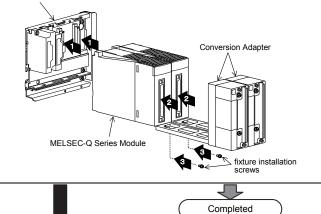
Install the MELSEC-Q Series Base Unit to the DIN rail.
