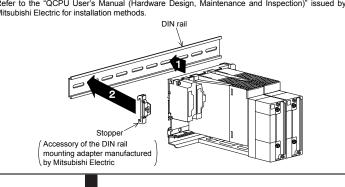
Install the stopper(right) to the Conversion Adapter DIN rail mounting bracket (right).
