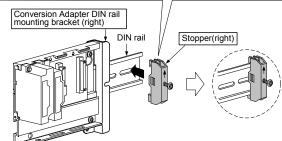
4. Check that the stopper(right) has been securely hooked on the DIN rail. Then slide it to the left side.
