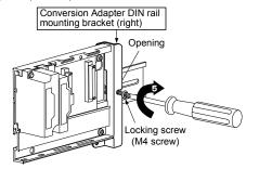
Mount the Conversion Adapter DIN rail mounting bracket (bottom) to the MELSEC-Q Series Base Unit and the Conversion Adapter DIN rail mounting bracket (right).
