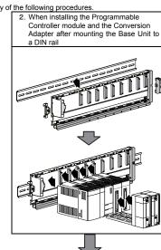
rail mounting adapter (large and small) manufactured by Mitsubishi Electric to the rear side of the MELSEC-Q Series Base Unit.
