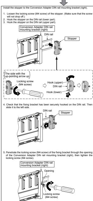
Mount the Conversion Adapter DIN rail mounting bracket (bottom) to the MELSEC-Q Series Base Unit and the Conversion Adapter DIN rail mounting bracket (right).
