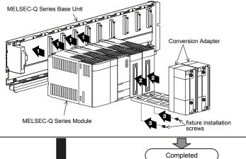
Install the MELSEC-Q Series Base Unit to the DIN rail.
