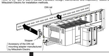
Install the stopper to the Conversion Adapter DIN rail mounting bracket (right).
